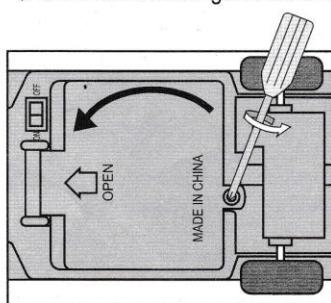
Unscrew the battery cover with a plus driver, press the buckle and open the cover.
